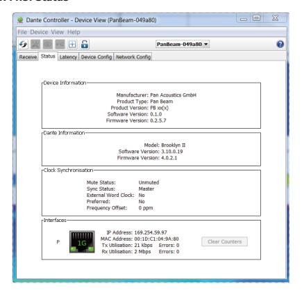
Via the "Status" tab, information on the device, firmware and software version, clock status and network interface can be called up.
