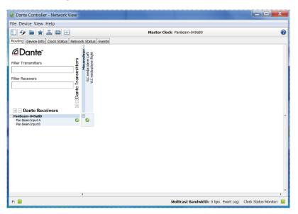
A Pan Acoustics loudspeaker appears in the Dante network under the "Dante Receivers" tab. The loudspeaker has two inputs, Input A and Input B.
