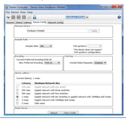
Various settings in the Dante interface of the loudspeakers can be made via the "Device Config" tab.
