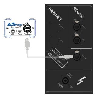
Each Pan Beam loudspeaker has an alarm contact. The loudspeaker can indicate a detected fault via this alarm contact. A switching relay is installed in the speaker for this purpose, which is closed in normal operating mode. If the loudspeaker has no supply voltage or if the DSP reports an error, the relay is opened.
