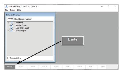
The loudspeakers in the Pan Beam series are to be set up through the Pan Beam Setup software. The Dante Controller software from Audinate must be installed to access a Dante network via the software. After successful installation, the Dante interface (Ethernet) appears in the footer of the Pan Beam Setup software.
