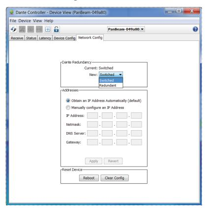
The Dante interface of the loudspeakers supports the "switched" and "redundant" modes in the Dante network.
