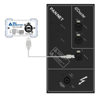
Each Pan Beam loudspeaker has an alarm contact. The loudspeaker can indicate a detected fault via this alarm contact. A switching relay is installed in the speaker for this purpose, which is closed in normal operating mode. If the loudspeaker has no supply voltage or if the DSP reports an error, the relay is opened.
